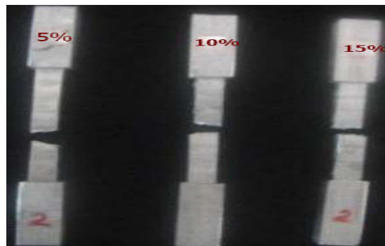
Figure: Tensile Specimens after test
